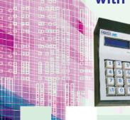
Each chamber will have terminal unit with Key Board & 16 Char. 2 line LCD display. It is connected with the Master controller. It displays last No. of token issued, Current Slot No, & Current Token No. On issuing of any new token, for the chamber and slot No, the display is up-dated. The key board has a master button I for calling in the next number.
