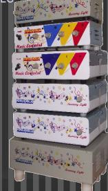
channel to 4 channel. These are manually controlled dimmers. 6 Channel dimmer has a master controller and action switch which can controls the lights in different modes.
